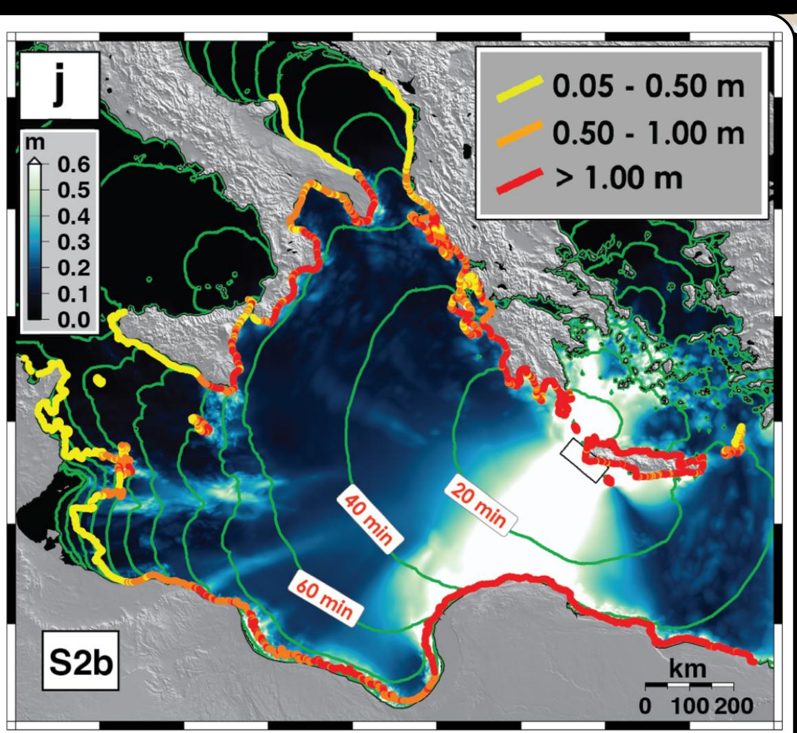
Maximum wave heights and tsunami travel time, Mw8, Hellenic Arc, from Basili et al. (2013)
